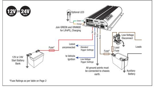
Figure 2.7.2 - Typical LiFePO<sub>4</sub> Setup
